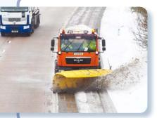
When freezing temperatures are forecast, the winter fleet will be out treating the roads with salt. The fleet includes new spreading vehicles which distribute the salt with less waste. During severe winter weather it is a round-the-clock operation to reduce the effects of ice and snow.
